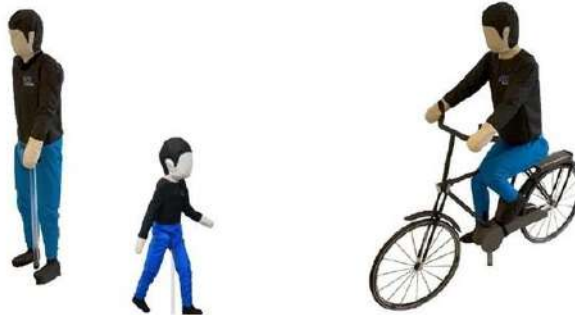
Images of Euro NCAP compliant adult, child, and bicyclist targets shown left to right (Source: Euro NCAP AEB document)
